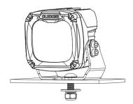
C.Loosen the fixing screws on both sides of the u-shaped bracket to adjust the angle of lamp, then fix it back
